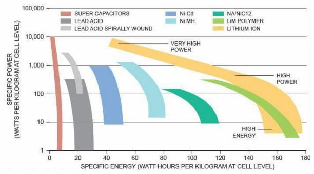
Figure 3.2 Specific power and specific energy of different battery chemistries (source Johnson Controls)
