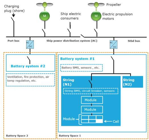
Figure B.1. Battery System and related sub-systems
