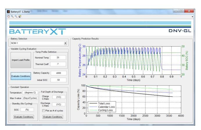
Figure D.2. Screenshot of Battery XT, showing user inputs which allow them to evaluate any chosen battery chemistry for any given application profile.
