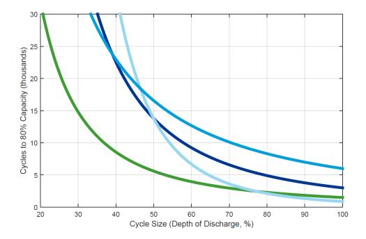
Figure D.1 Batteries are able to perform more cycles when only a small portion of the total energy is used in each cycle – a nonlinear relationship that varies substantially between different battery chemistries and manufacturer.
