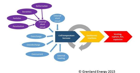
Figure 5.1 Overview of factors that can cause unwanted temperature increase on cell level in a battery system (Grenland Energy)
