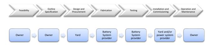
Figure 4.1. The battery system in the shipbuilding process and the responsible party
