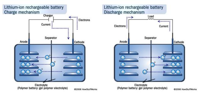
Figure 3.3 Basic principles and components of a lithium-ion battery
