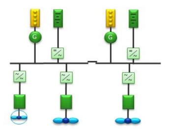
Figure 3.9 Battery hybrid propulsion
