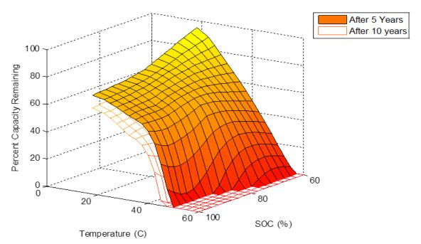
Figure 3.5. Evaluation of expected capacity shows the detrimental effect of high temperature and high SOC on calendar (standby) loss
