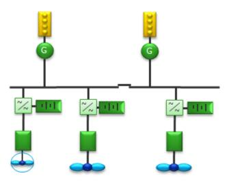
Figure 3.10 Hybrid battery propulsion with distributed batteries
